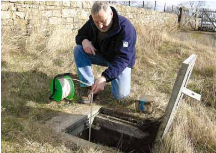
Dipping a farm borehole, Newton of Falkland, Fife
