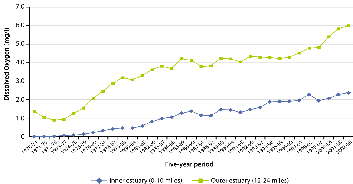
Figure 4: Dissolved oxygen levels in the Clyde Estuary, 1970-2006, as five-year mean values (as 95th percentile)
