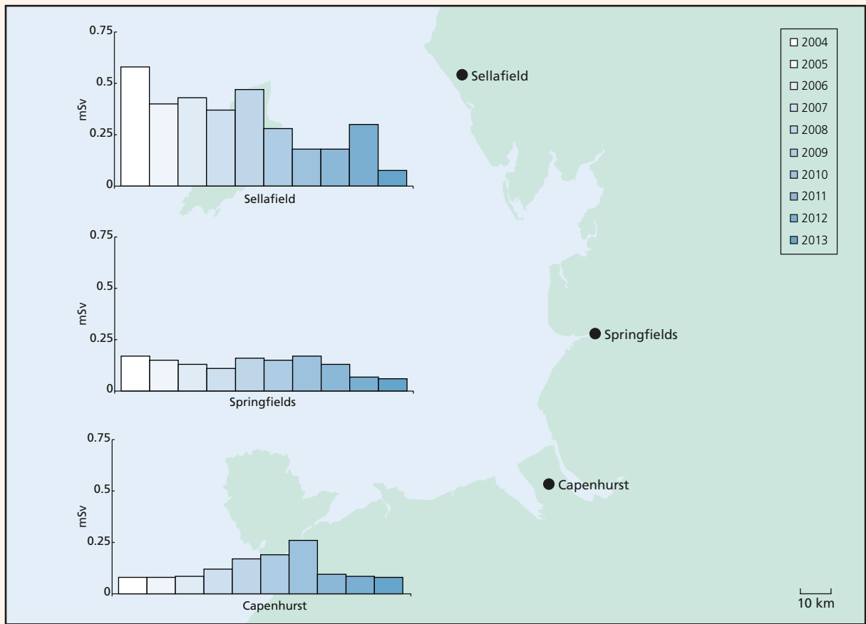
Figure 2.1. Total dose due to operations, nuclear fuel production and reprocessing sites, 2004-2013 (Exposures at Sellafield receive a significant contribution to the dose from technologically enhanced naturally occurring radionuclides from previous non-nuclear industrial operations)
