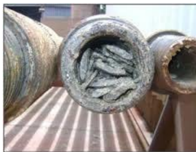
Used drilling pipe showing contamination
