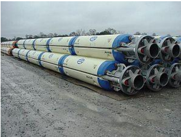
Unused production risers
